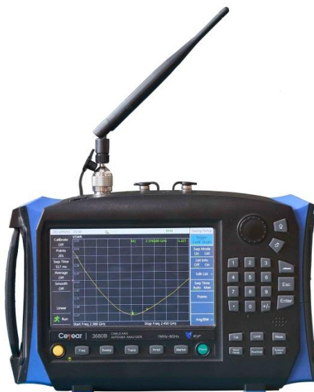
Antenna return loss/VSWR measurement
